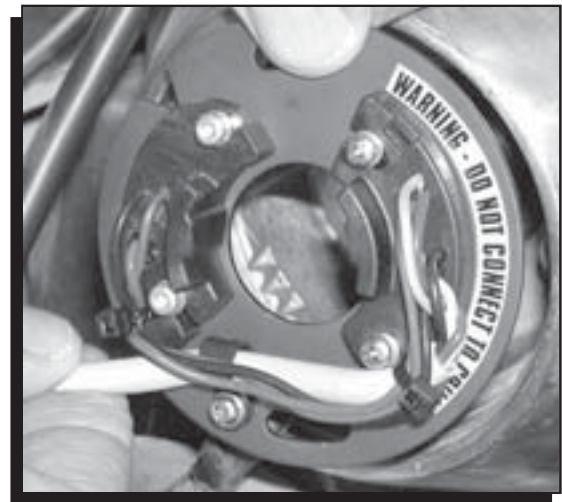
Figure 1 Installing the MSD Pickup Assembly.
